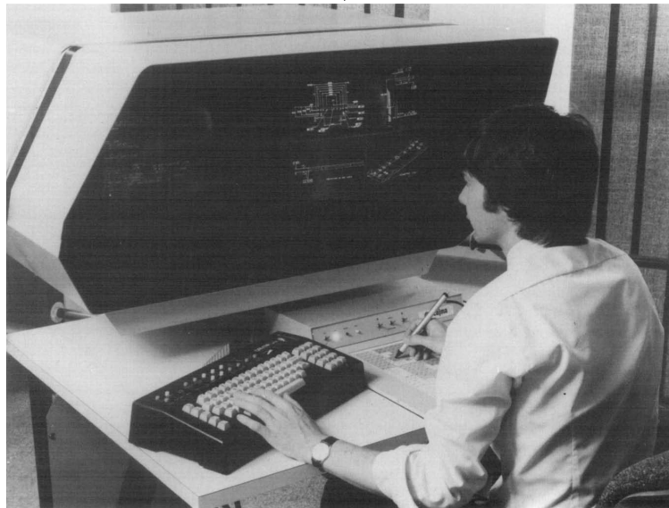
Fig. 1.7: Workstations used during the development of integrated systems during the early years of CAD/EDA. a) Two workstations used in Texas Instruments circa 1970 [43]. The left workstation, used for schematic design, is equipped with a large interactive screen and stylus. The right workstation is used for layout drawing and is equipped with a large interactive screen and a small additional display. b) IC design workstation during the mid-1980's used to generated the layout of an IC [44].
