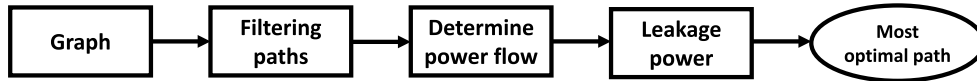
Fig. 2. Flowchart of the proposed methodology. A graph of the system is initially generated. Paths connecting the initial and final states of the process satisfying the constraints are determined. The power flow within the system is subsequently evaluated to determine the total power consumed by the system. The optimal system is based on the total power consumption and delay of each path.
