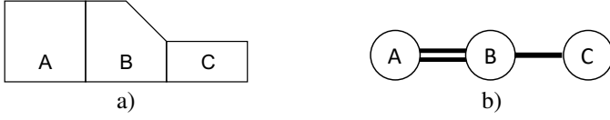
Fig. 6. Conversion of irregularly shaped tiles into an equivalent graph. a) Tiles A and B have a twice wider contact than tiles B and C, and b) nodes A and B have double conductance as compared to nodes B and C.
